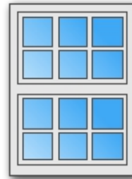
Double Hung with Grids Grids Can Be In One or Both Sashes
